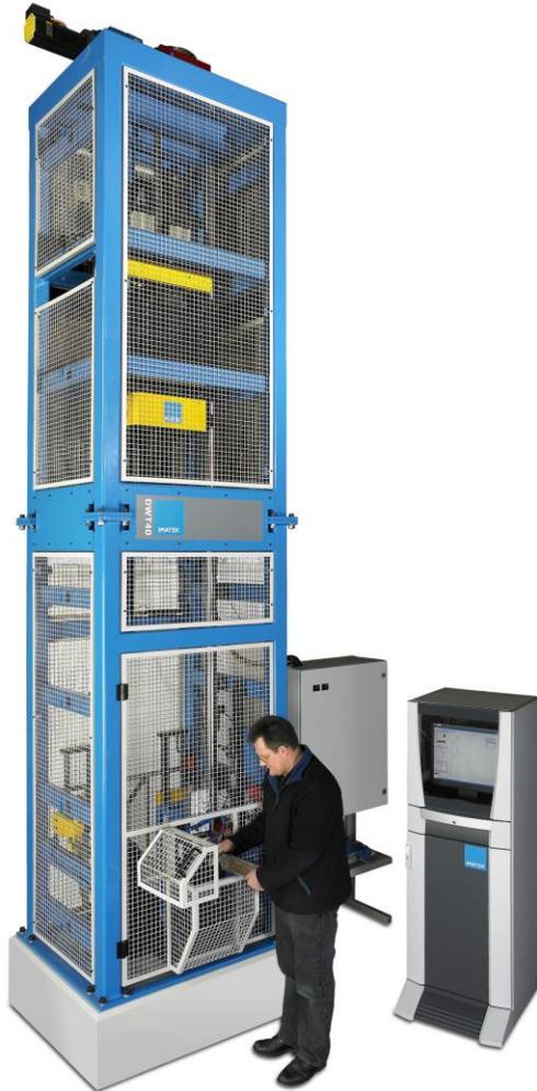
A drop weight impact tester for measuring the fracture characteristics and fracture ductility of steel specimens according to the following standard:
