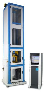
A range of impact test systems designed for dynamic compression testing. To characterise energy absorption, cushioning performance, resilience and fatigue at varying rates of strain. Used both in R&D environments and for quality control.
